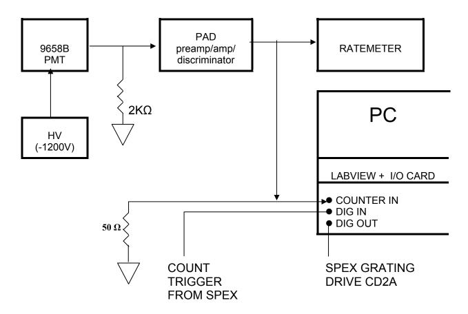
The specifications of the 9658B are shown in Figs. A5-3,4; note that the bias voltage to the cathode is always negative, and the <u>maximum cathode bias HV = -2300 V.</u>
